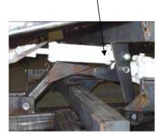
Position and/or rotate the rod clamping fasteners away from the bracket mount to prevent damage to the fastener
