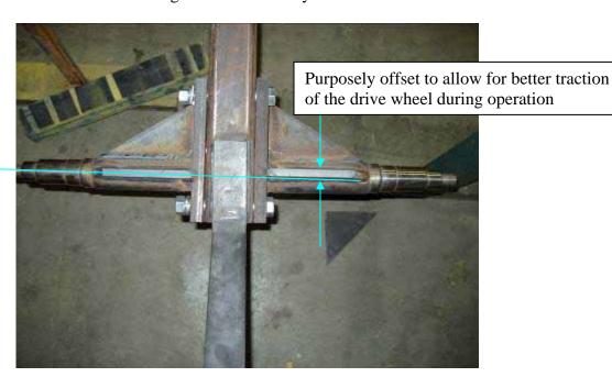
3) Install wing frame wheel legs using 8116-802 (1-1/4" x 3-5/8" NC bolt w/Nylock Nut), 6136-627 bushings, and 7896-250 machine bushings.
