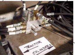
Main Hydraulic Manifold – to be attached to main tongue weldment
