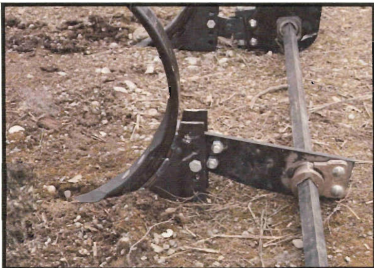
Replaceable, high chrome cast wear parts, easy-mount shoe
